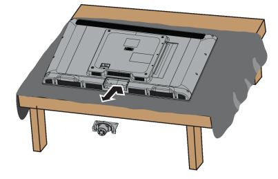
4 Attach the wall-mount bracket to your TV using the mounting holes on the back of your TV. See the instructions that came with the wall-mount bracket for information about how to correctly hang your TV.
